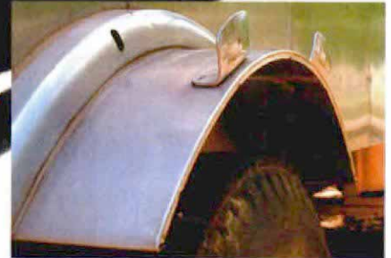
Reclaimed soap dishes double as hooks. These wheel covers are actually stainless-steel shower fixtures acquired during a renovation.
